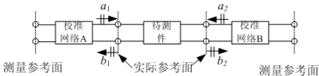
FIG. 2 Block diagram of S-parameter test system for two-port network
