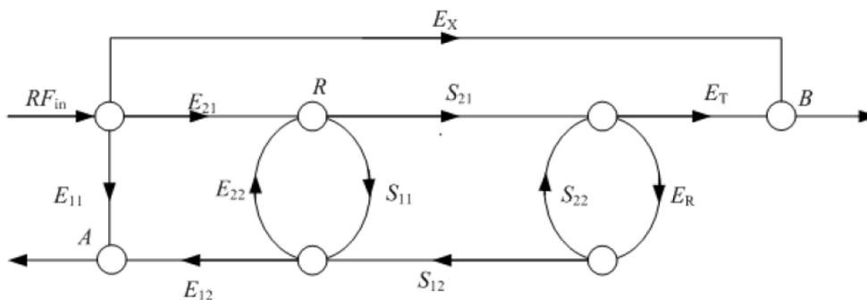
FIG. 3 describes the systematic error of the S-parameter test system using a 12-item error model. (Here is the forward error, the reverse error model is similar)
