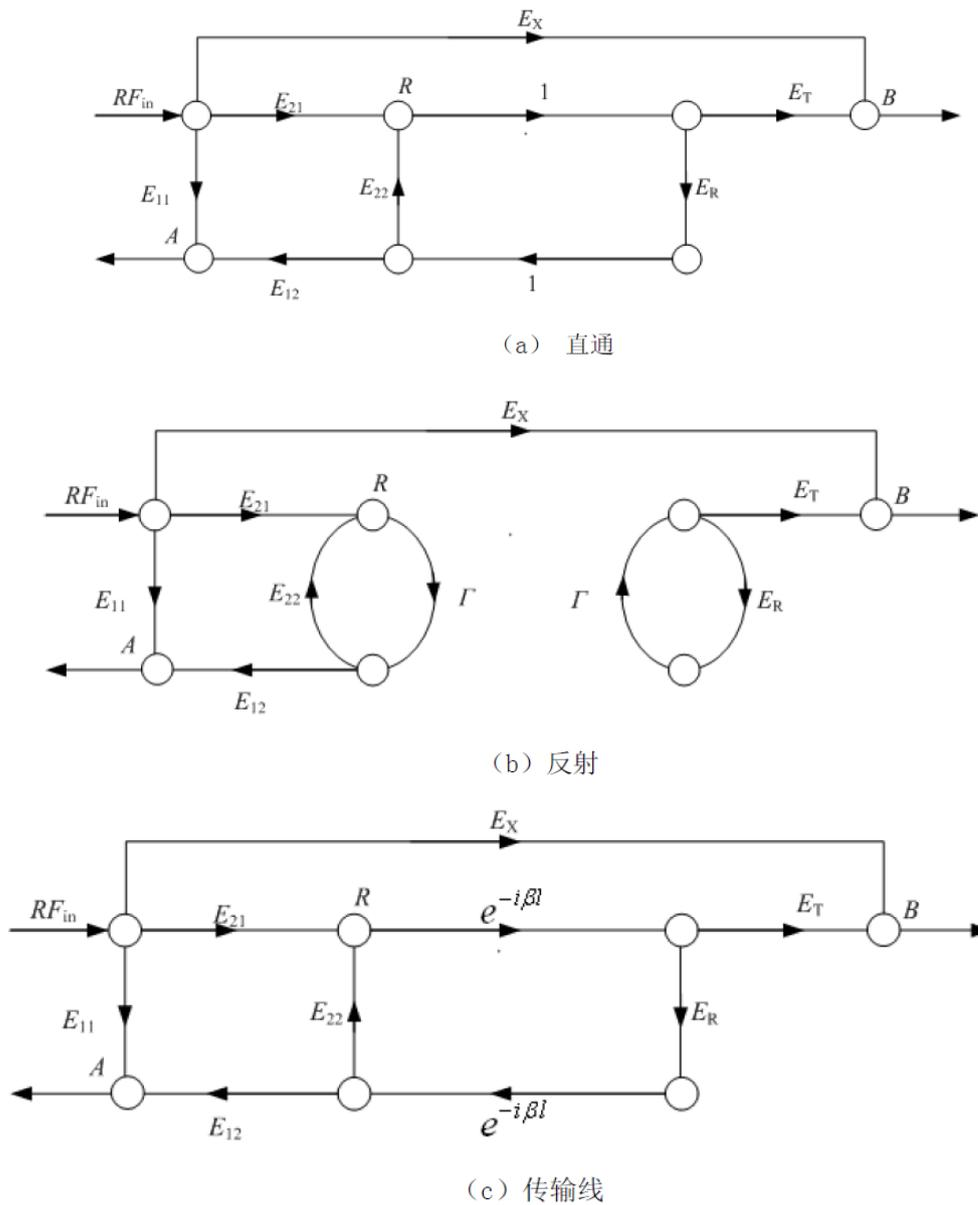
Figure 4 Signal flow diagram of straight-reflection-transmission line calibration method
